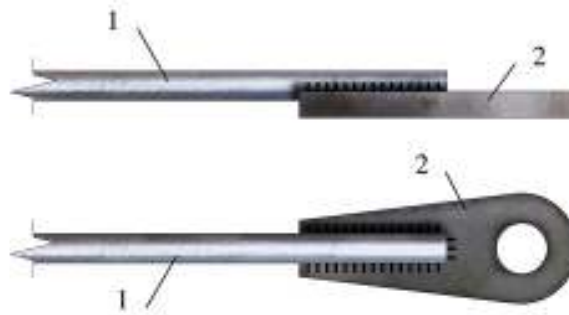
Fig. 8. The ends of the bottom chords: 1 – steel rod, 2 – steel drop plate with a hole
